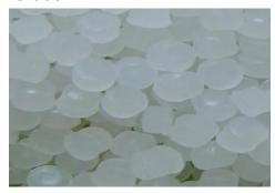
Middle melt viscosity, suitable for extrusion molding.
