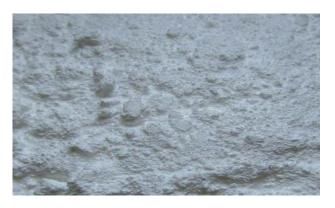
T-1 PVDF for coatings is solid powder, it can mixed with acrylic resin, additive, and become superior performance baking PVDF fluorocarbon coatings. Compare with other grade of PVDF, T-1 is more suitable for stoving finish, baking light color coatings.
